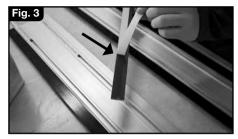
STEP 3. Peel away the backing from the new Guide Strips (Fig. 3).
