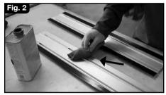
STEP 2. Clean the track using rubbing alcohol before installing new Guide Strips (Fig. 2).
