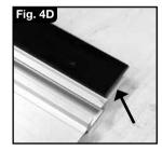
STEP 4. Align the new Guide Strips flush to the end of the track with the arrows (Fig. 4A & Fig. 4B). Position the Guide Strip against the shoulder and press the new Guide Strip down on the track (Fig. 4C). The Guide Strip will be slightly shorter than the track end (Fig. 4D). Re-install the starting block in the end of the track, and refer to Accu-Cut<sup>™</sup> manual for calibration.
