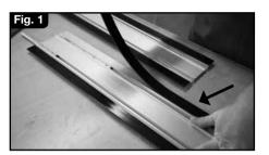
STEP 1. Remove the Starting Block from the track. Remove the used Guide Strips (Fig. 1)
